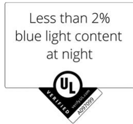
Figure 1. The UL Verification Mark that indicates lighting fixtures that minimize circadian disruption at night
